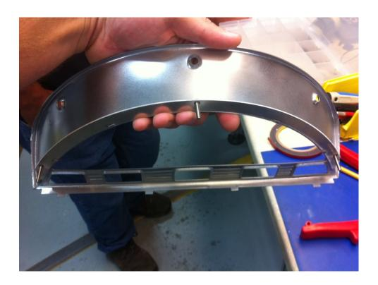
5. Install the bezel/bracket assembly over the cluster. Line up the three machine screws with the holes in the lens, diffuser, and housing. The tabs on the lower edge of the bezel will go in slots on the top dial.
