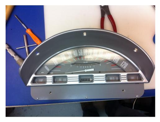
6. Complete the assembly with three 6-32 nuts (N0632UZ) on the backside of the cluster. Tighten them with a  $\frac{1}{4}$ " nut driver.
