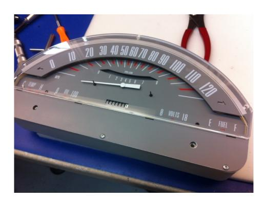
3. Use needle nose pliers to bend the five top tabs on the bezel as shown below.
