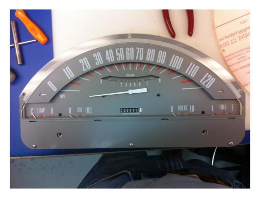
2. Remove the protective paper film from the lens (LEFT56) and clean it with a soft cloth and Windex. Use compressed air to remove any dust from the cluster and place the clean lens on top of the diffuser.
